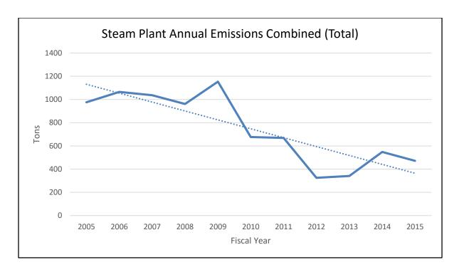
The steam plant annual emissions combined are estimated by applying formulas from the U.S. Environmental Protection Agency (EPA) to coal and natural gas inputs at the Steam Plant. Currently, there is no measuring device employed "at the stack." The Knoxville campus applied to the Knox County Department of Air Quality Management for UT Knoxville's original's Title V permit in 1999.
