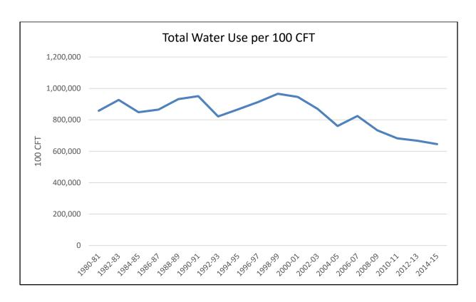
This chart illustrates the consistent decrease in water usage per student and campus square footage that is largely attributed to the university's push for installing water reducing/reusing technologies such as low flow installations, waterless urinals, and cisterns.
